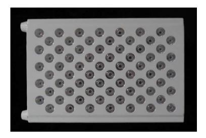
Irradiance measurements acquired with LLIA Asset #A049 - International Light Technologies Model ILT950 Irradiance Meter System with FFO600SC/A2/W cosine response input optic. Irradiance measurements taken in the LightLab goniophotometer room with stray light reduction. Test subject was allowed to reach stabilization according to IES LM-79-19 criteria prior to measurements. Luminaire was measured in laboratory conditions.
